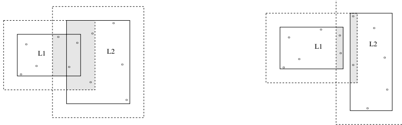
(a) Overlapping MBRs ( R tree and R^* tree) (b) Non-overlapping MBRs ( R^+ tree)
